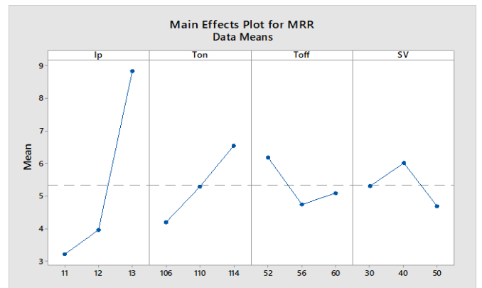
Fig. 2. Main effect plot for MRR for Brass wire
