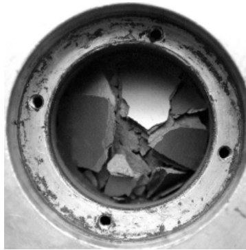
Fig. 2. Briquette destroyed as a result of an outburst induced under laboratory conditions
