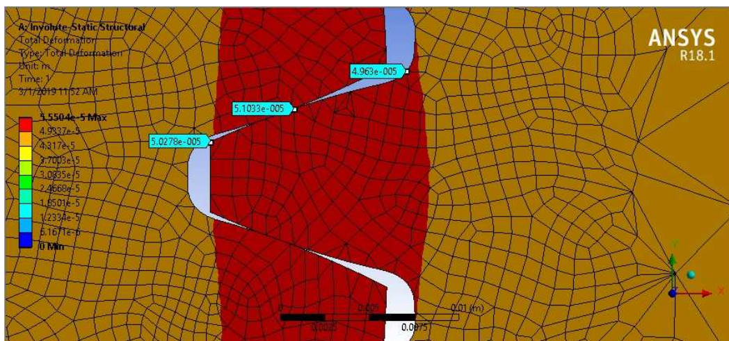
Fig. 6. Deformation results of the modified tooth profile.
