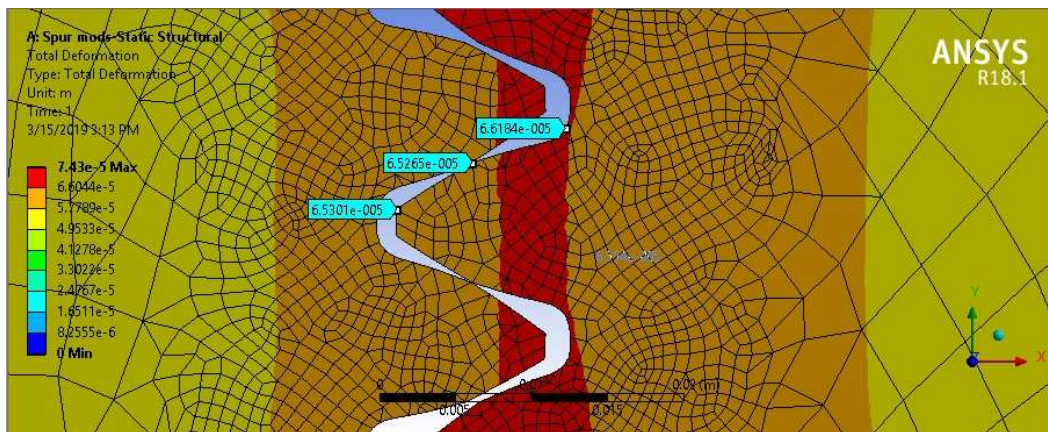
Fig. 5. Deformation results of the involute tooth profile.
