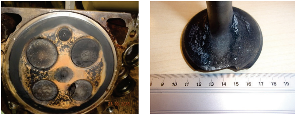
Fig. 1. View of partially burnt valve sockets in the engine cylinder head and valve heads
