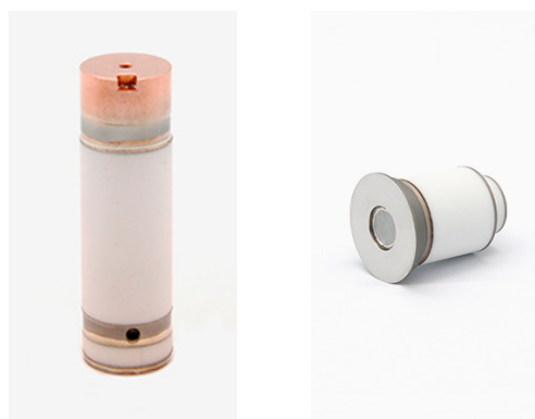
Fot. 9. Lampy z CNT firmy VSI Medical: z lewej lampa o dużej dawce (50 kV, 50 mA, Ø20×68 mm), z prawej lampa do jonizatora (5-15 kV, 3-1,5 mA, Ø34×34,35 mm)[7] Photo 9. VSI Medical CNT tubes: on the left a high-dose lamp (50 kV, 50 mA, Ø20 × 68 mm), on the right, an ionizer lamp (5-15 kV, 3-1.5 mA, Ø34 × 34.35 mm) [7]
