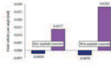
Fig. 18. Final vehicle body yaw angle during the manoeuvre
