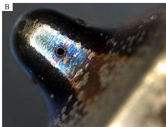
Fig. 7. Tip of the damaged piezoelectric injector: a) appearance after removing b) appearance after clearing – visible discoloration caused by the impact of high temperatures
