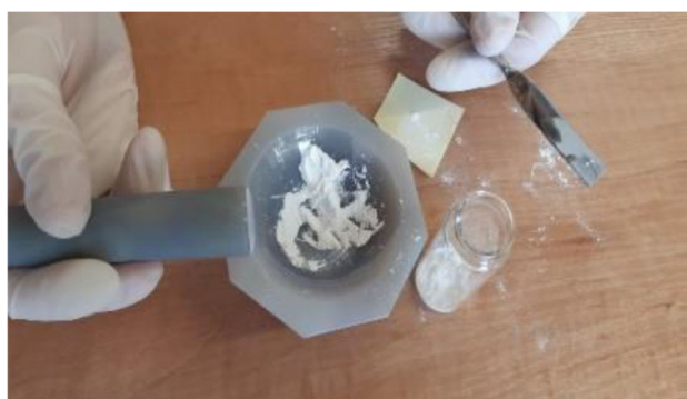
Fig. 3. The TiO 2 nanopowder obtained after grinding in an agate mortar
