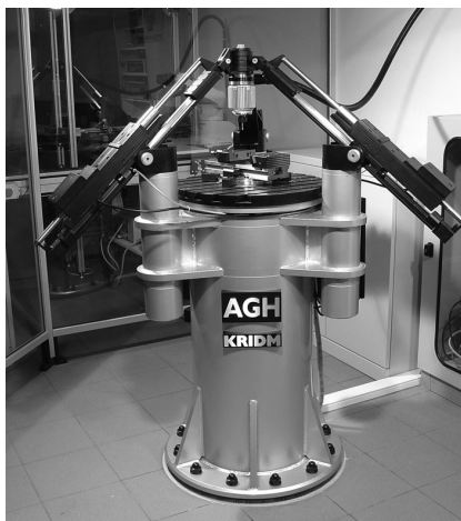
Fig. 1. Parallel robot with three degrees of freedom for milling
