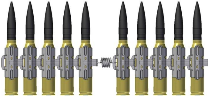
Fig. 9. Ammunition belt (link considered to be a spring element)
