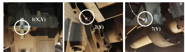
Fig. 2. An example of the implementation of measuring points on the drive system [phot. Of authors]
