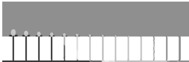
Fig. 8. Air velocity on the inlet side of the machine – 0.01 m/s
