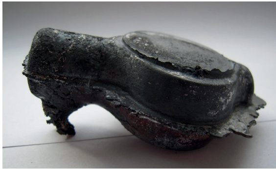
Fig. 9. Picture of die stamping of steel 100Cr6 (ŁH15) shaped at 1400°C in the semi-solid state
