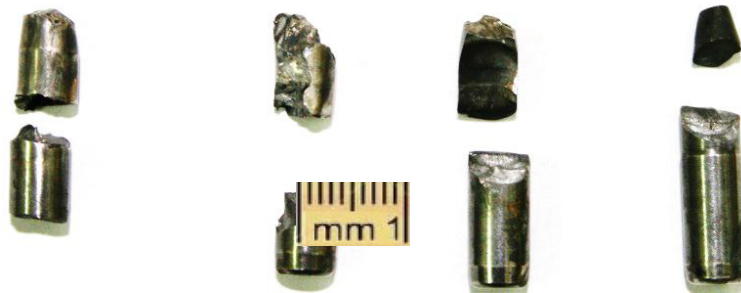
Fig. 24. Bullet core after 60° oblique perforation tests
