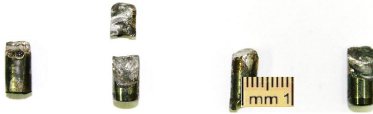
Fig. 21. Bullet core after 50° oblique perforation tests
