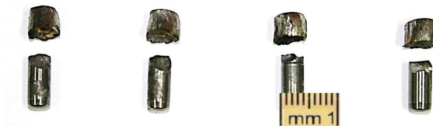
Fig. 14. Bullet core and resulted plugs after normal perforation of 6 mm thickness plates
