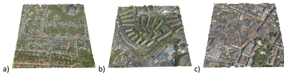
Fig. 3. LiDAR measurement data presented in the form of RGB colour point clouds for a fragment of a single-family housing estate (a), a multi-family housing estate (b) and the city centre (c) in Bydgoszcz
