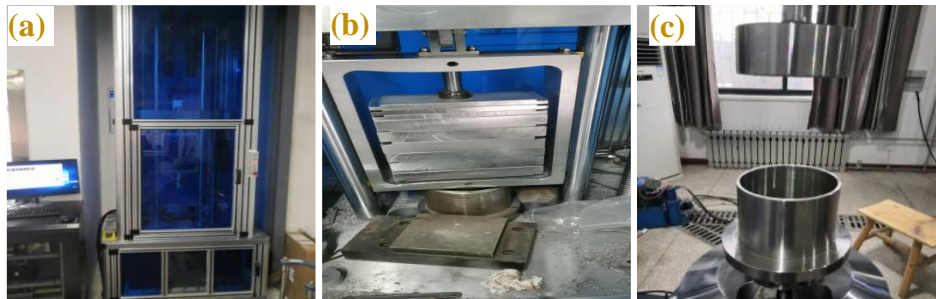
Fig. 4. Ore breakage test system;(a) drop weight impact equipment; (b) particles recovery unit; (c) particle group test tank
