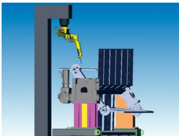
Fig. 3. Simulation of correct interaction of a standard robot (ArcMate 100iC/7L) with a frame-type (flat) manipulation object model mounted on an "H" positioner and ensuring vertical orientation of the electrode axis
