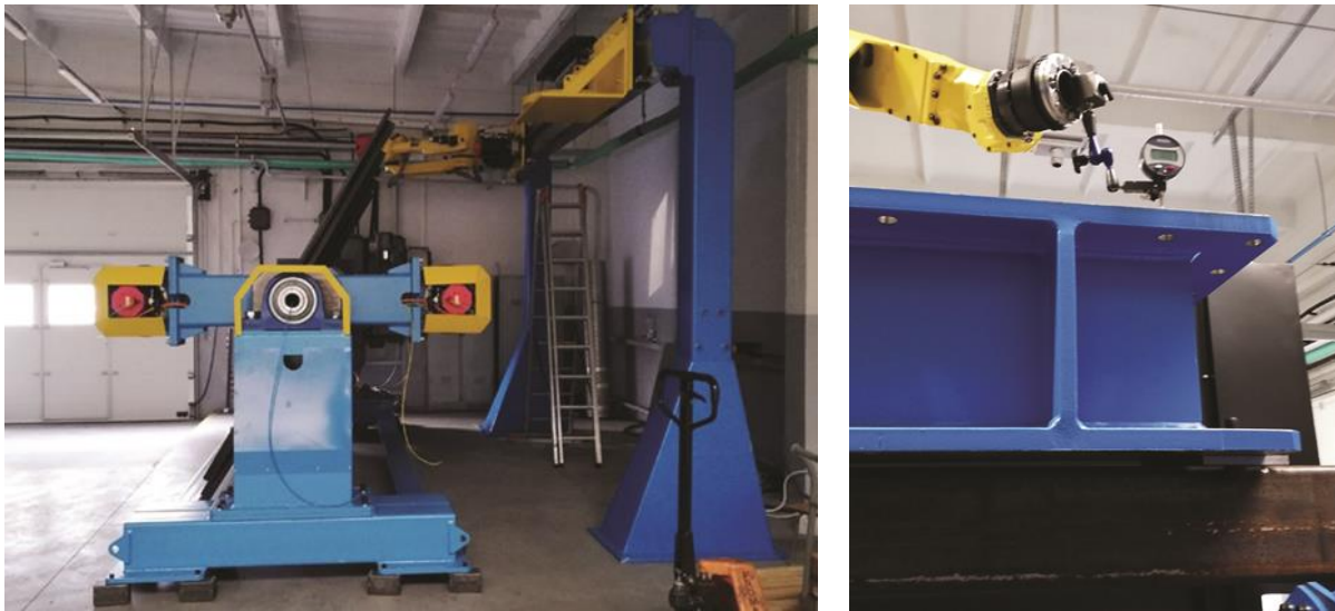
Fig. 14. Prototype gate runway with additional module for transporting accessories during assembly phase
