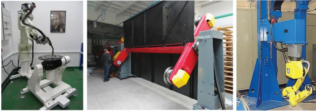
Fig. 1. Examples of external axes of industrial robots: a) two-axis positioner with Kawasaki FA006E robot in the laboratory of the Department of Welding Engineering, b) two-axis "H" type positioner, ZAP Robotics, c) cantilever with vertical robot locomotion, ZAP Robotics
