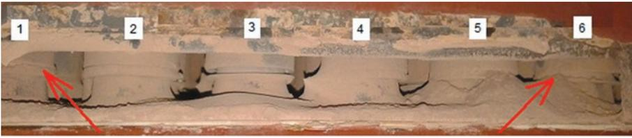
Fig. 15. Cyclone outlet gaps after supplying 2150 g of dust at dust extraction rate of  $m_0 = 5\%$  – view from the dust extraction manifold: 1, 2, 3, ..., 6 – consecutive number of the cyclone in the column (arrow indicates the cyclones with gaps clogged with dust)
