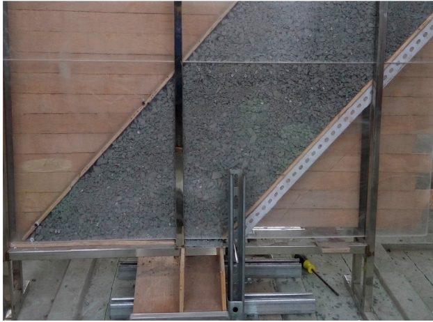
Fig. 1. Scaled physical model for ore draw under inclined wall boundary condition
