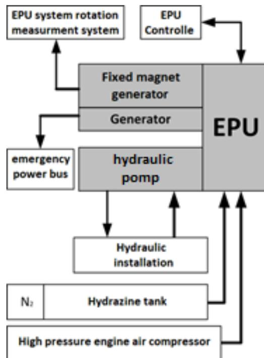
Fig. 1. A functional diagram of EPU system of emergency power supply EPS of F-16 multirole aircraft
