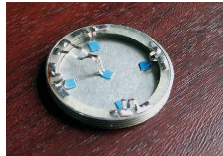
Fig. 8. Membrane element with temperature-sensing elements
