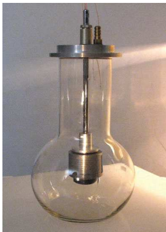
Fig. 17. Vacuum flask with membrane elastic element
