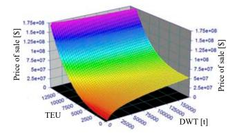
Figure 3. Projecting the price of a container ship depending on the DWT capacity and TEU capacity according to formula (4)
