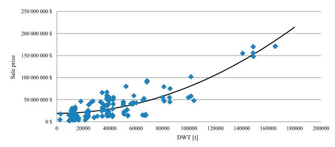
Figure 2. Approximations of container ship price depending on DWT capacity. Relationship (3) in comparison with reference data
