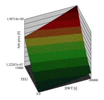
Figure 5. Projecting the price of a container ship depending on the DWT capacity and TEU capacity according to the formula (5)
