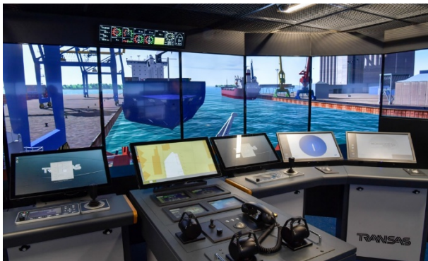
Figure 1. The main bridge of the navigation simulator at SAMK, Rauma
