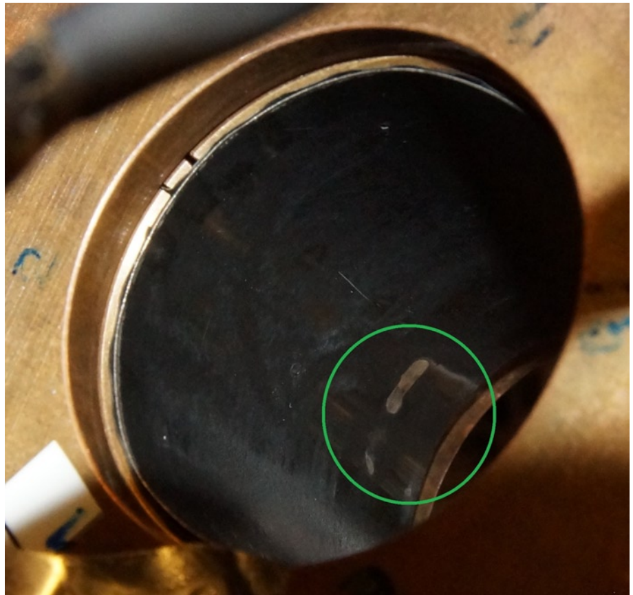
Fig. 2. Abrasion of the sputtered protective layer on the inner surface of the GFB's top foil
