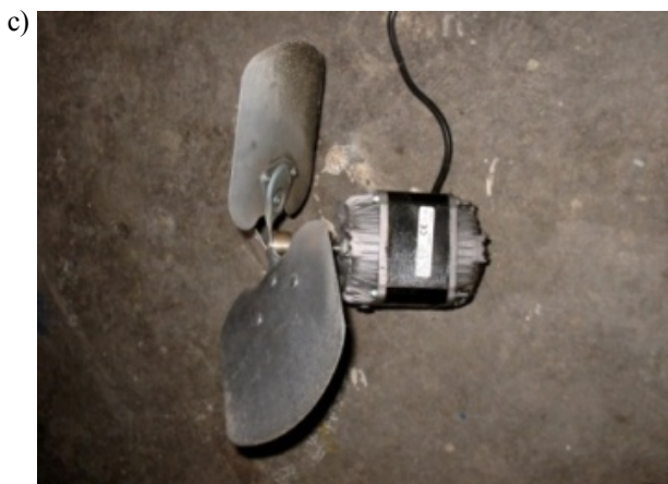
Fig. 1. Examples of refrigerating system component faults: a) refrigerant leaking from a refrigerating installation, b) damage to a compressor, c) damage to a condenser fan [4]
