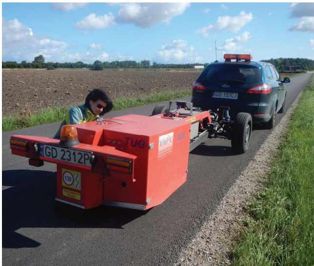
Fig. 5. Test trailer R2 Mk.2 built by the Technical University of Gdańsk
