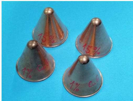
Fig. 1. Dimensions and photo of shaped charge liners made with the use of the sintering method
