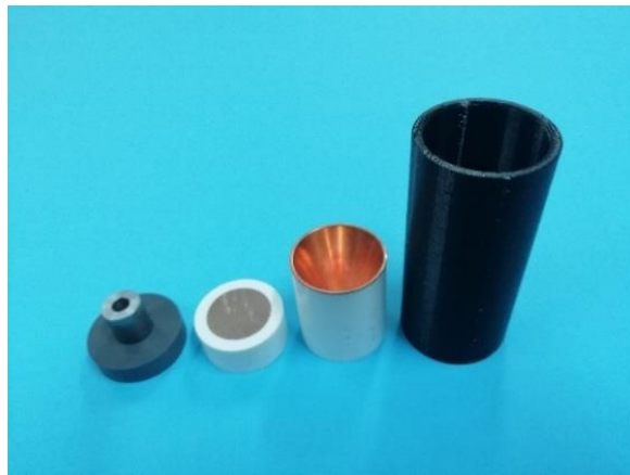
Fig. 3. Components of the shaped charge system used for recording the jet
