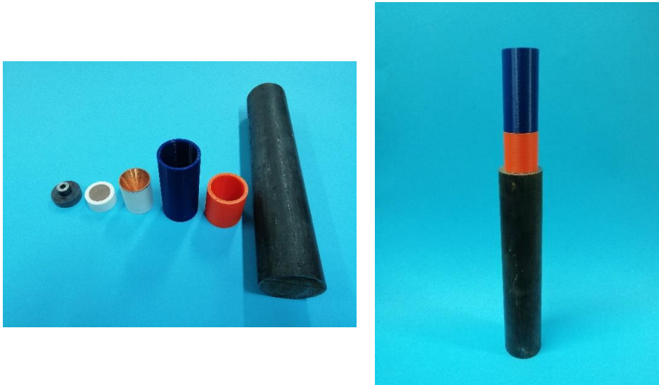
Fig. 5. Images of the components and the complex system used for testing the steel penetration depth of the shaped charge jet
