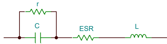
Fig. 3b. Electrical Equivalent Circuit of an Aluminium Electrolytic Capacitor
