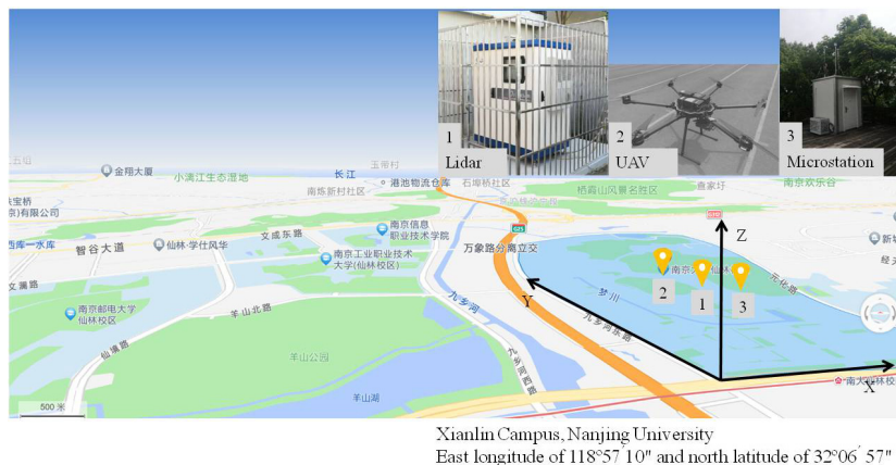
Fig. 4. The diagram of field experiments including location and observation instrument.
