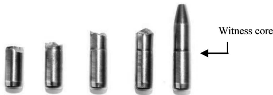
Fig. 5. 7.62 mm AP bullet core after shot tests
