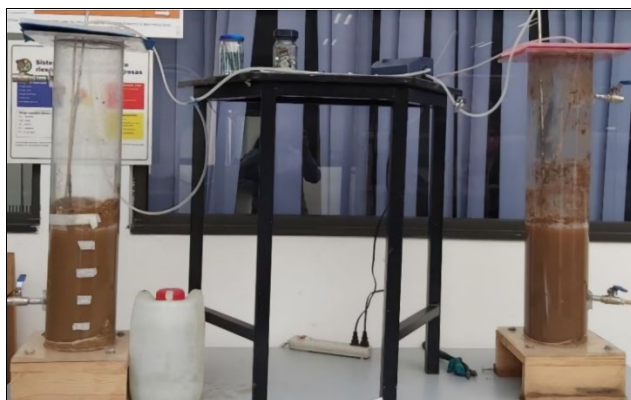
Fig. 1. View of equipment for SBR operation
