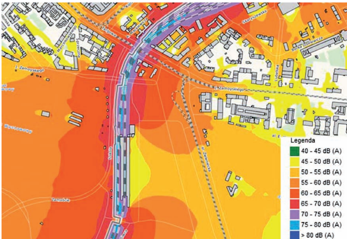
Fig. 2. Example map of a railway line with noise level distribution (isolines) [49]
