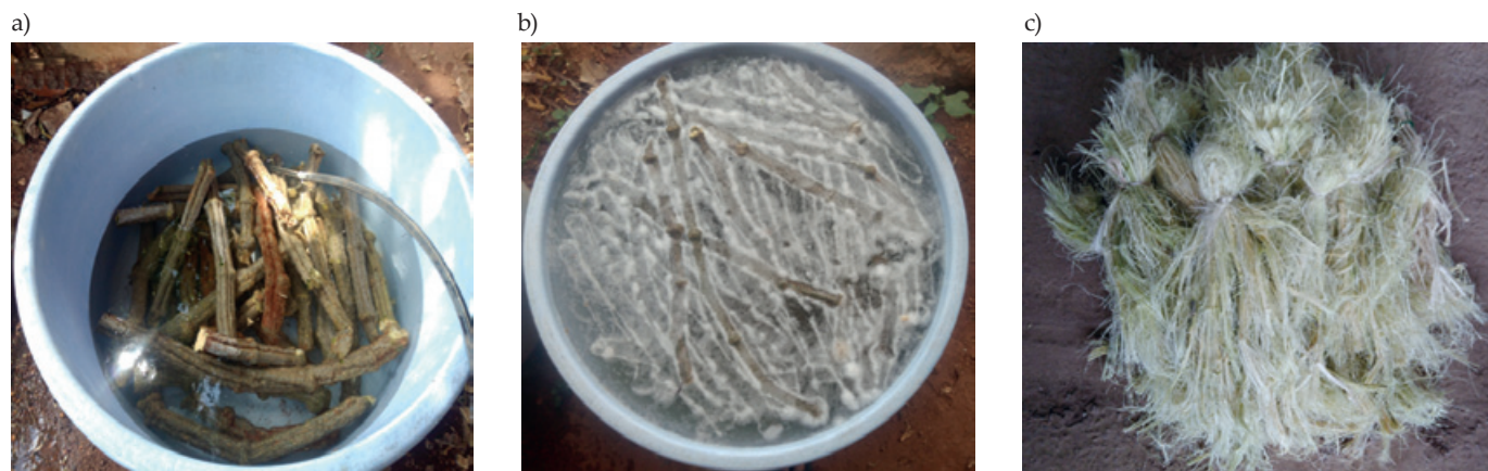
Fig. 1. Fiber extraction: a) CI sliced and immersed in water, b) immersed CI after 3 weeks, c) extracted CI fibers
