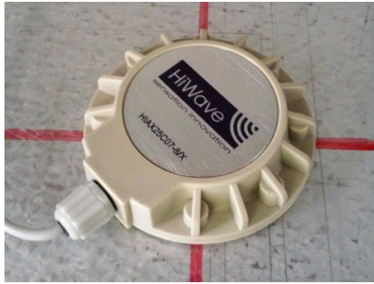
Fig. 3. A photograph of an actuator mounted to the casing.
