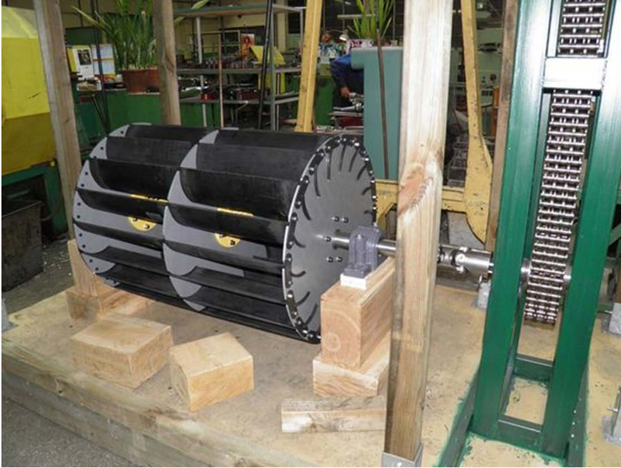
Fig. 2. Turbine rotor, installed [Włodzimierz Sawicki, 2010]
