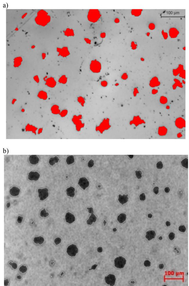
Fig. 7. An image of the microstructure of the analysed cast iron with marked graphite particles selected for the measurement ( $D > 10\mu\text{m}$ ): a) light microscope b) X-ray microtomograph (tomogram)
