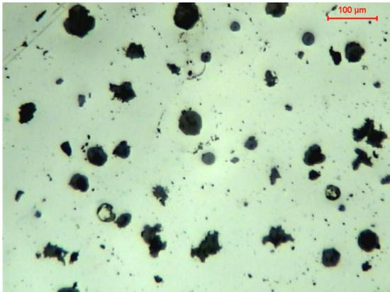
Fig. 3. Microstructure of ductile iron, unetched metallographic specimen
