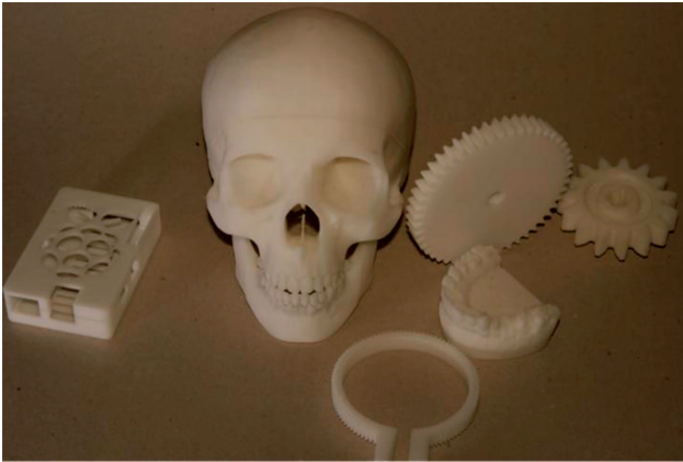
Fig. 1. Sample models printed by FDM method
