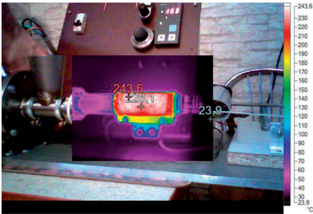
Fig. 3. Extruder visible in FLIR thermal imager
