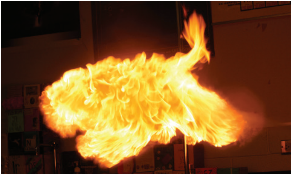
Fig. 1. Fire of a cloud LPG with the air – flash fire
