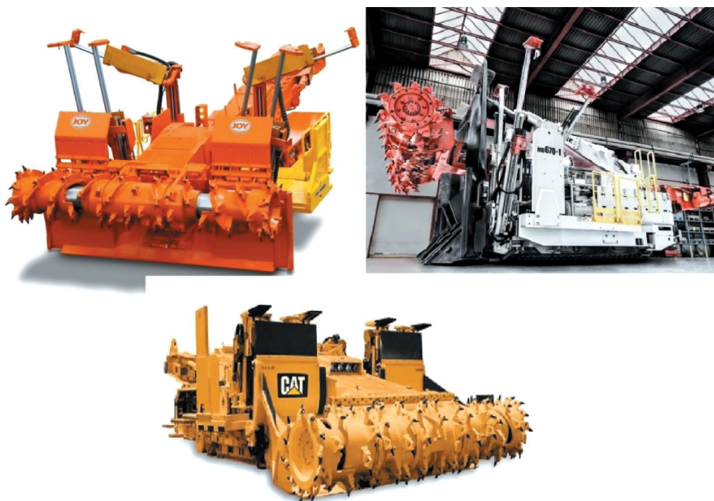
Fig. 2. Bolter miners produced by Joy 12CM30, Sandvik MB670 and CAT CM845 [22–24]
