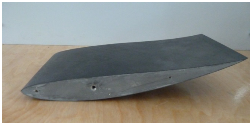
Fig. 4. A model of a wing section used during the first experiment
