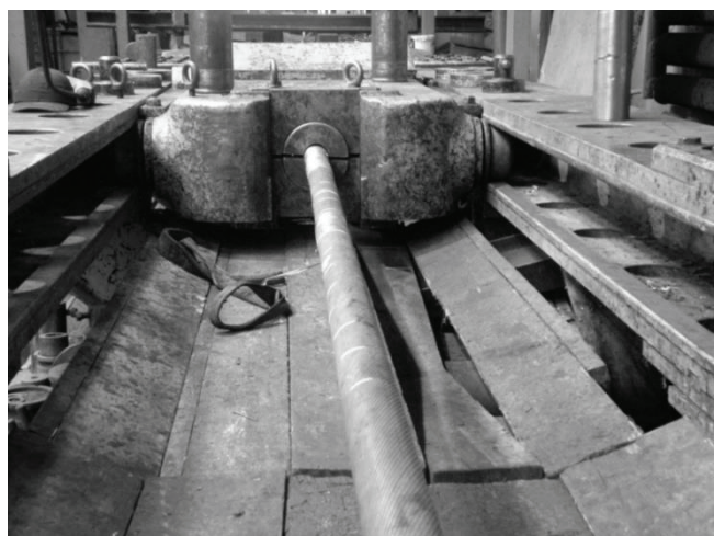
Fig. 2. Stand for testing cables
