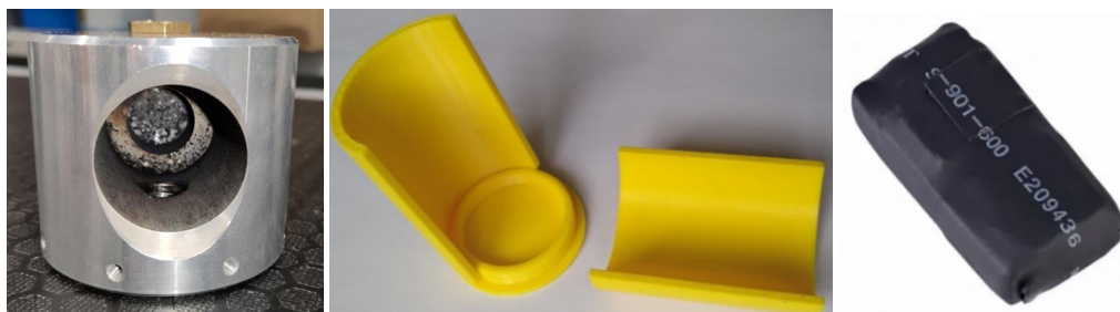
Figure 1. Ejector body (left), load housing (centre) and ejected Global Positioning System (GPS) locator (right)
