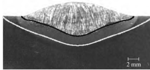
Fig. 14. Comparison of numerical results and image of metallographic section: black and white lines correspond to the calculated fusion line and the calculated temperature limit of the full transformation of austenite A_3 , respectively
