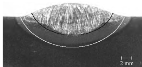
Fig. 10. Comparison of numerical results and image of metallographic section: black and white lines correspond to the calculated fusion line and the calculated temperature limit of the full transformation of austenite A_3 , respectively
