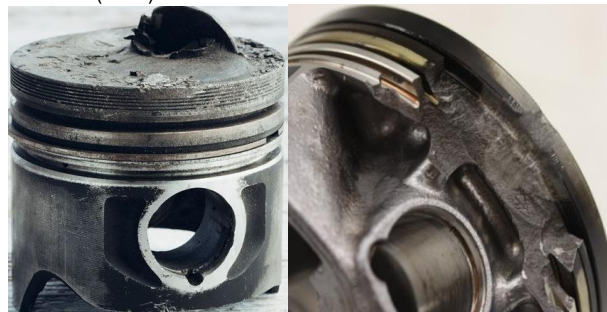
Fig. 3 Example of piston damage due to LSPI
