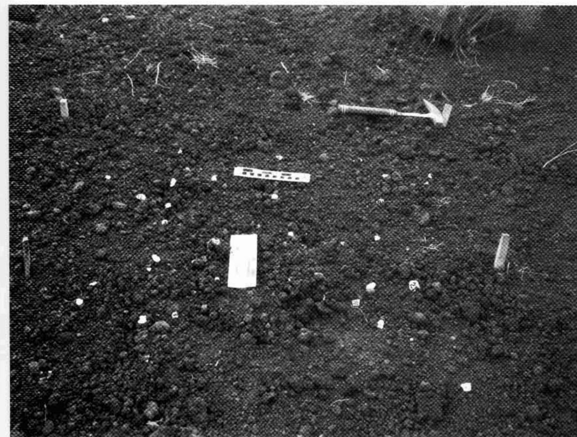
Fig. 2. Selected photographs of the experimental grids. Each cinder was originally placed 10 cm from its neighbor (field rulers and rock hammer for scale). (a) Grid 1 on August 4, 1992, showing movement of white-painted cinders and two grooved disturbances across one corner of the grid. Uphill is to the top of the photograph. (b) Grid 2 on August 16, 1994, showing 25 months of particle movement. Uphill is to the top of the photograph. (c) Grid 3 on August 17, 1994, showing several considerable changes. Downhill is to the top of the photo-
