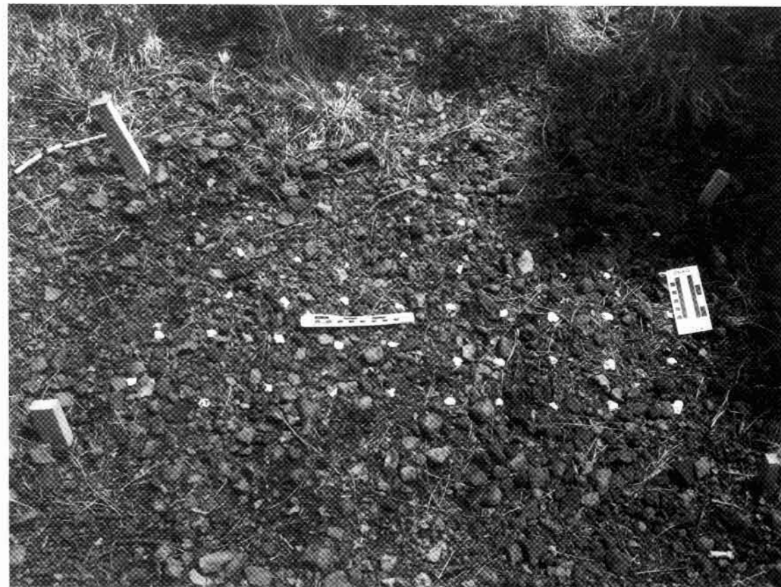
graph. Two corner stakes are lying on the ground near their original positions, another is hidden from view against the handle of the rock hammer, and the fourth is missing. Note the small log or branch washed into the confines of the grid and the large log 1.5–2 m downhill from the bottom of the grid. The smaller log obscures an animal burrow located near it. Sediment has accumulated beside the larger log. (d) Grid 4 on August 17, 1992, showing a minimal amount of movement after one month. Note the tree shadow and the coarse grain size of the surrounding cinders. Uphill is to the top of the photograph.
