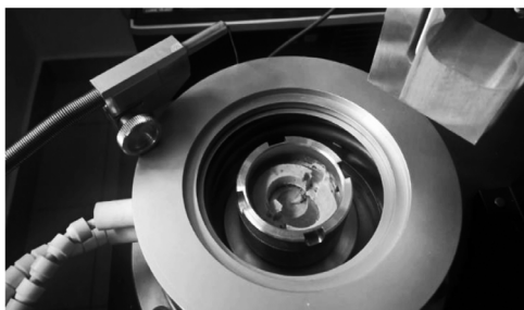
Fig. 9. Example of a sample destroyed during testing, Pd – 90°
