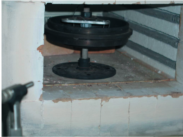
Fig. 3. Test stand for natural frequency determination of the brake drum – drum placed in the oven
