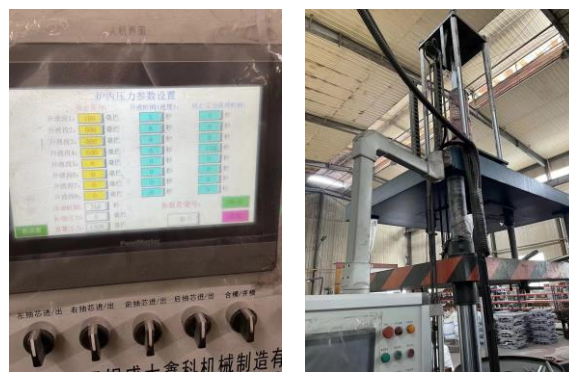
Fig. 13. Low-pressure casting equipment and actual parameter settings
