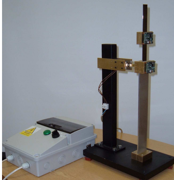
Fig. 4 Experimental model for verification of dynamic damping
