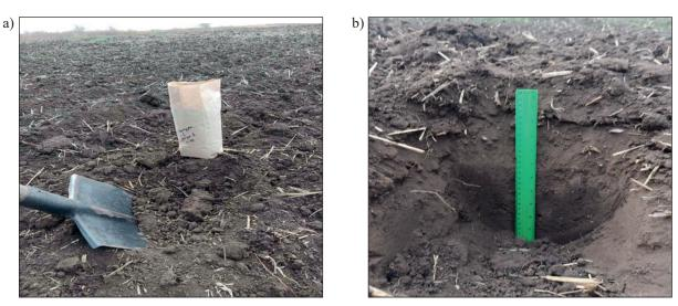
Figure 2. The technology of soil sampling: a) the first sage; b) - the second stage
